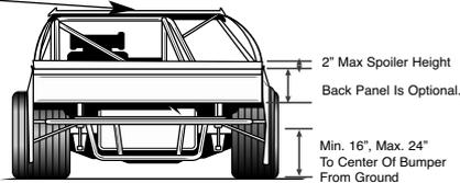
78" Maximum Body Width At Bottom Of Panels Near The Ground.
