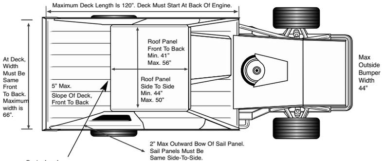
Back of roof can be curved forward a maximum of 2 inches.
