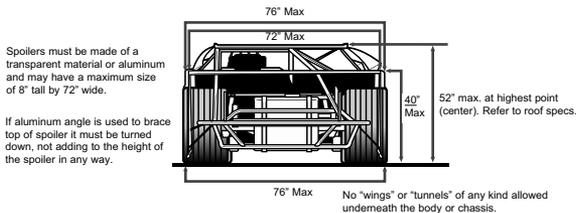
40" after the race, measured at the center of the deck from left to right.
